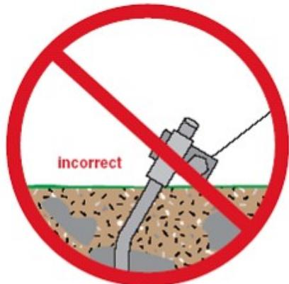
**WARNING:** Rock anchors can fail under high wind loads if they are not installed into solid rock. Rock surface must be within 1" of the rock anchor tension head in order to prevent failure. Rock anchor drive rods must be installed into predrilled holes not to exceed 3/4" diameter.
