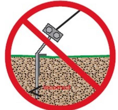
**WARNING:** Ground anchors can fail under high wind loads if they are not installed to their full depth, resulting in severe damage to the home.
