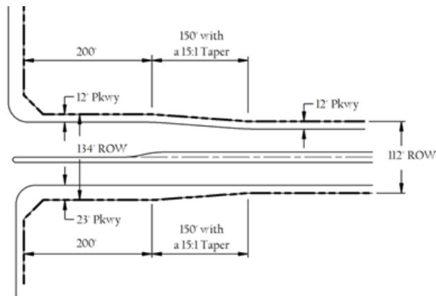
Figure 22. Typical Roadway Dimensions Approaching Major Roadway Intersections
