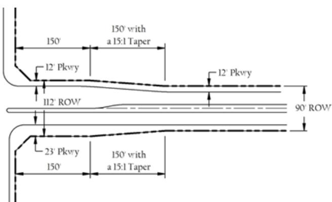
Figure 23. Typical Roadway Dimensions Approaching Minor Roadway Intersections
