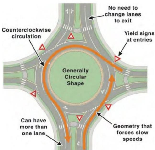
Figure 24. Roundabout Elements
