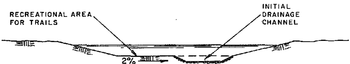
RIPRAPPED INITIAL DRAINAGE CHANNEL WITH OVERFLOW FOR MAJOR DRAINAGE RUNOFF
